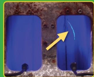
Same view, crack easily observed with the "Crack Finder" penetrant and UV light.
